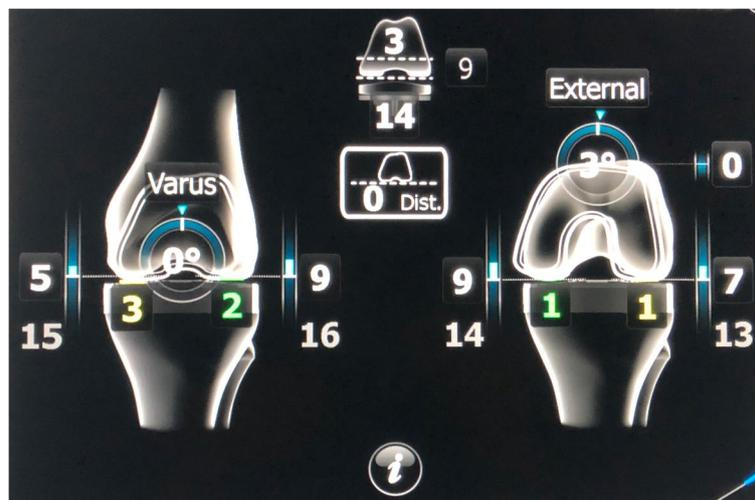
**Fig. 4** Screenshot displaying customization of femoral component in order to obtain desired gap balance in extension (left) and 90° flexion (right). One can customize femoral size, depth of distal femoral resection (joint line), orientation of distal femoral cut in coronal (varus/valgus) and sagittal (flexion/extension) planes, femoral rotation, and insert size
