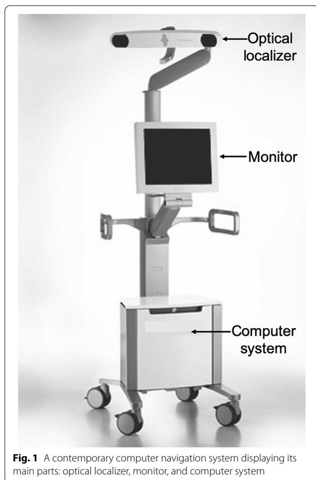
**Fig. 1** A contemporary computer navigation system displaying its main parts: optical localizer, monitor, and computer system
