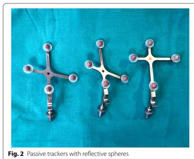
**Fig. 2** Passive trackers with reflective spheres
